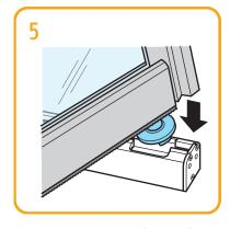
• Insert swivel bearing (258801) of the swivel panel through the opening in the floor rail.
